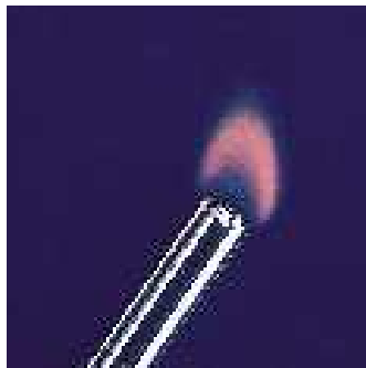
Hydrogen burning in air to form water.
