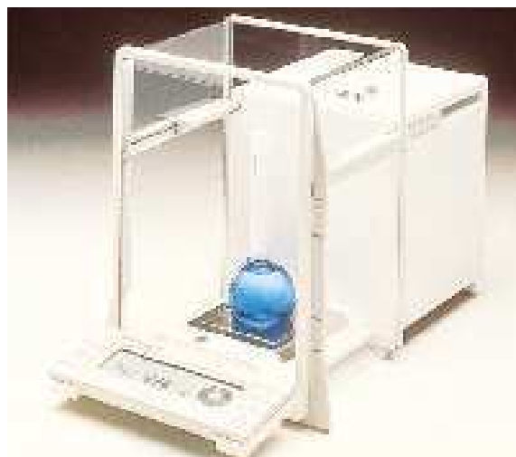
FIGURE 1.11 A single-pan balance.
